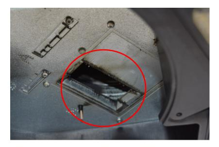
Turn on the exhaust and check that the 'door' opens wider – that might make it easier to clean.
